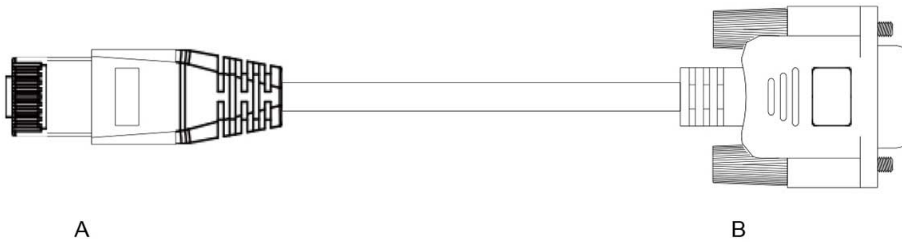
Figure 3-15 PC Communication Cable Appearance Example
