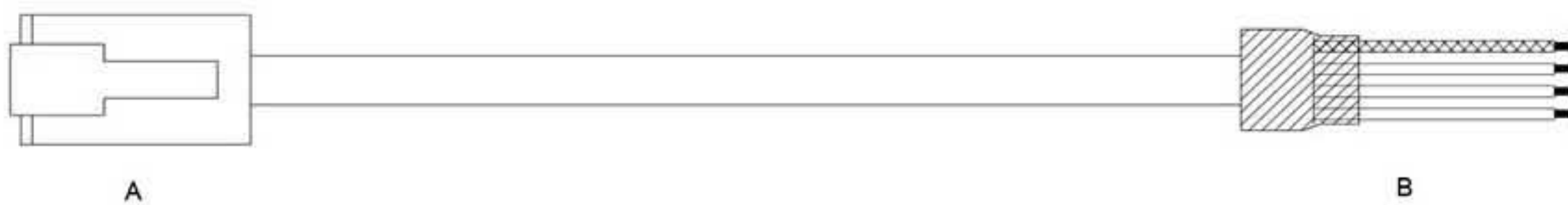
Figure 3-7 Appearance example of PLC and servo communication cables
