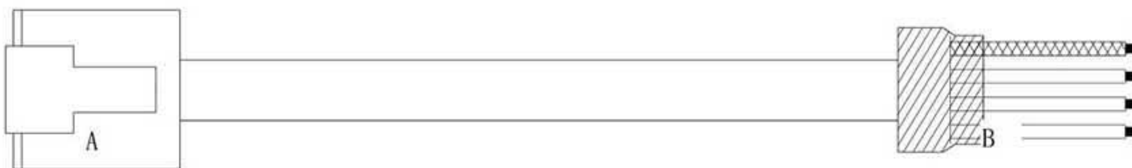
Figure 3-11 Appearance example of PLC and servo communication cables
