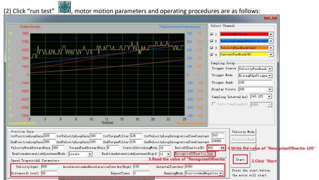
The value of the load inertia ratio obtained from the above steps can satisfy most applications, but for some cases where the load inertia is very high, the value of Pr0.04 can be increased to more than 1000.
